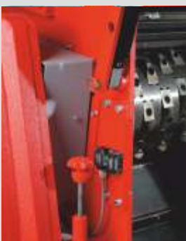
Safety unit for use on the exposed screen basket
